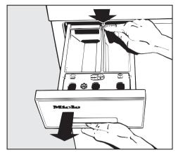
Press down the red release catch and at the same time pull the drawer right out of the machine.
